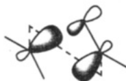
Interaction of the \sigma and a substituent \pi orbital upon inward rotation.
